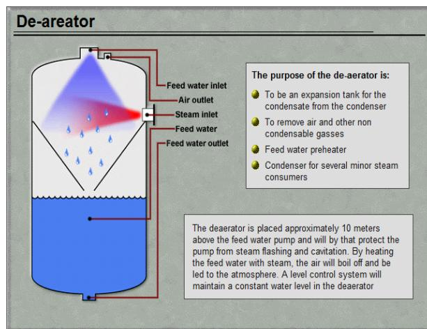
This is a device whose function is to heat the water filling the boiler as well as to remove the gases contained in the water condensate. The deaerator heats the water by mixing the water with used steam so that the hot fresh water will rise and emit gases from the air exhaust pipe / water outlet.
